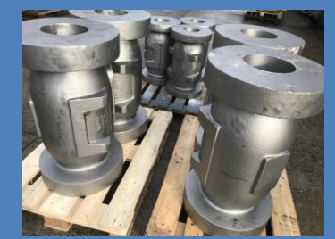
DIFFERENT MATERIAL OF CASTING THE VALVE BODY, FROM CARBON STEEL, STAINLESS STEEL INCLUDED SUPER DUPLEX
