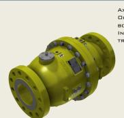
AXIAL CHECK VALVE **DN 150\_PN 160** DPERATING WITH COMPRESSED AIR, VALVE BODY FROM CARBON STEEL CAST, INTERNAL FEEDBACK SYSTEM WITH LINEAR TRANSMITTER 4-20 MA
