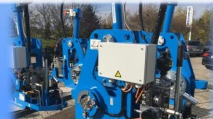
Automatized damping unit HSAU16 mounted on butterfly tilting check valves DN700
