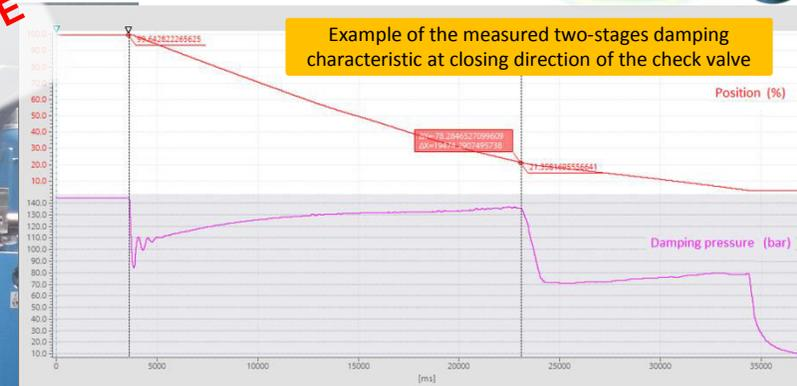
Before delivery each damping unit type AHSAU is tested on HYDROMAT® Torque Test Station at *real operating torques and times*:
