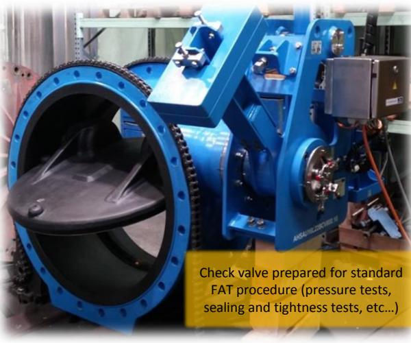
Check valve prepared for standard FAT procedure (pressure tests, sealing and tightness tests, etc...)
