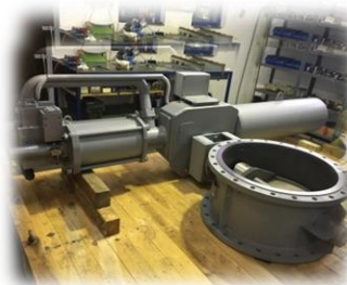
Actuator with the valve is tested and ready for delivery from HYDROMAT factory
