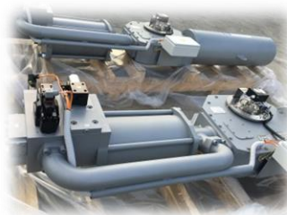
Actuator with the valve is tested and ready for delivery from HYDROMAT factory
