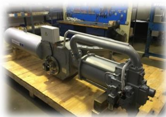
Actuator with the valve is tested and ready for delivery from HYDROMAT factory
